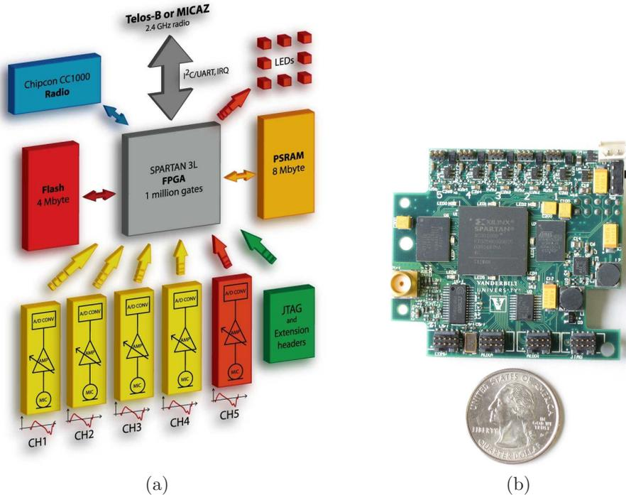
**Figure 1.** (a) Multi-channel Sensor board Modules and Architecture, (b) New Sensor Board 2.
