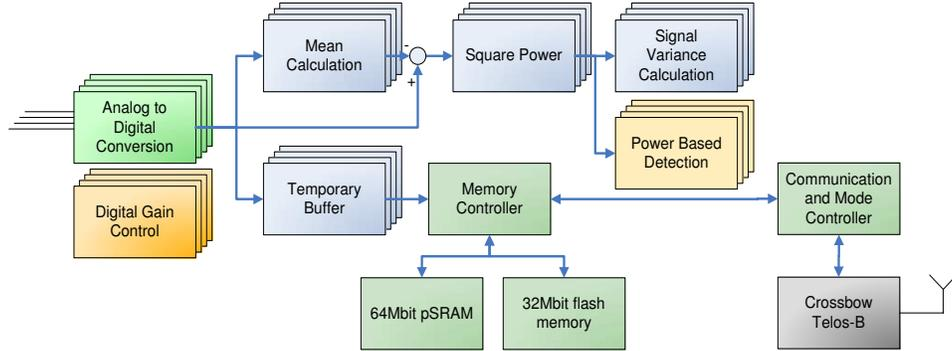
**Figure 4.** Block diagram of transient detection application
