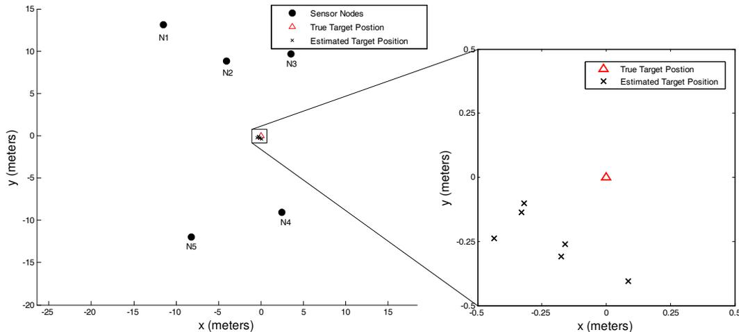
**Figure 7.** Plot showing the deployed sensor nodes, the true target position and the estimated target location. Also shown is the portion of interest around the true target position.
