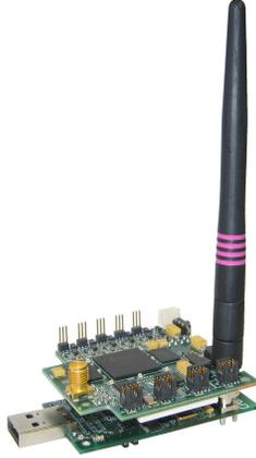
**Figure 5.** A sensor node - consisting of Telos-B mote and Sensor Board 2
