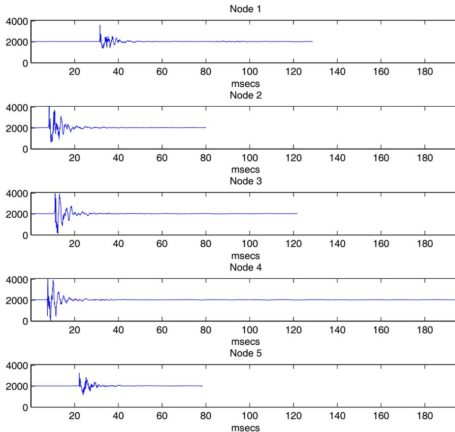
**Figure 6.** Acoustic data of the detected event in the five nodes.
