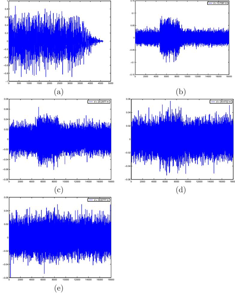
**Figure 2.** (a) The original 20mm gun fire acoustic signature and the received signals of different sensors for (b)  $d_{1,s} = 10.7381\text{m}$  (c)  $d_{2,s} = 20.2977\text{m}$  (d)  $d_{3,s} = 29.4732\text{m}$  (e)  $d_{4,s} = 39.6777\text{m}$ .
